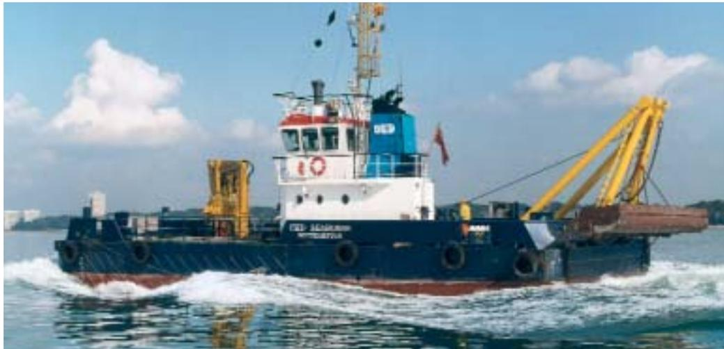
UKD Seahorse is a 25 metre Multicat designed specifically by Damen Shipyards for UK Dredging. She is specified to provide a multi-purpose dredging support vessel with bed-levelling, buoy handling and survey capability.
