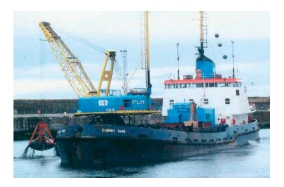
A self-propelled grab hopper dredger, Cherry Sand has recently been modernised with a Pulleman grab crane and equipped with a range of buckets to enable dreging in a wide variety of materials. The hopper well is fitted with a grid to avoid debris being deposited at sea, and discharges via hydraulically operated bottom doors.
