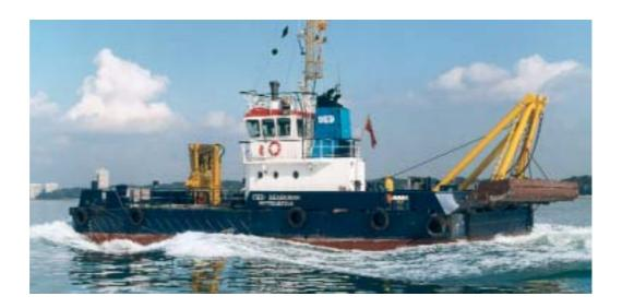
UKD Seahorse is a 25 metre Multicat designed specifically by Damen Shipyards for UK Dredging. She is specified to provide a multi-purpose dredging support vessel with bed-levelling, buoy handling and survey capability.
